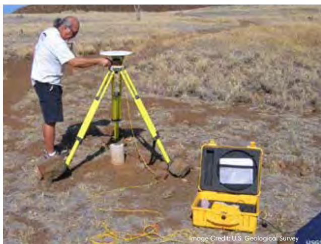
setting up a portable GPS receiver on a Hawaiian volcano
