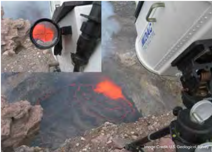
measuring volcanic gases with a spectrometer at Kilauea Volcano, Hawai'i
